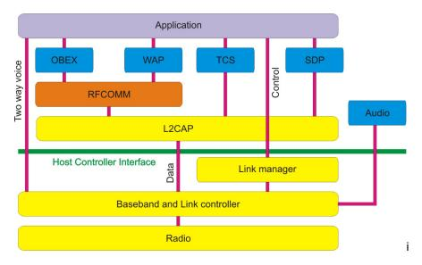
The basic process is simple: raw data at the top needs to be converted into bits and bytes that can be transmitted via radio signal and built back up into the raw data the application at the other end can work with.
