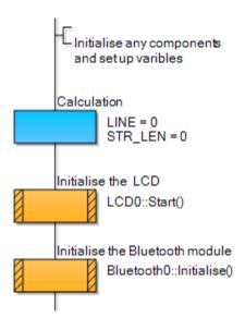
The basic program flow is to start off by initializing any components and setting up any default variable values. Add in an LCD Start macro, and a Bluetooth Initialize macro.
