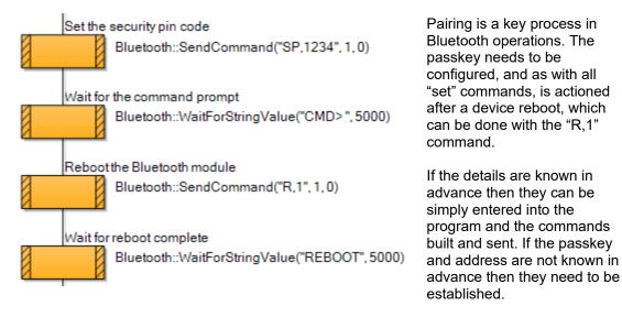
The Bluetooth device address can be obtained by downloading the BT\_TEST Flowcode program. You may wish to note down the addresses for the various boards.
