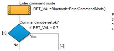
For example, here we test the return value to check that command mode was successfully entered.
