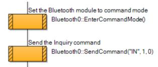
Before a command can be sent to the Bluetooth module, it needs to be put into command mode with the EnterCommandMode function of the component.
