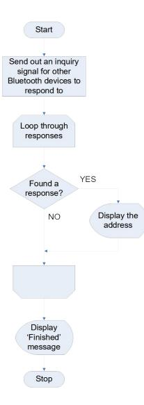
The plan is to send out the inquiry signal, then to loop through checking for any responses, displaying the address of any device that responds, and the completion message once the inquiry is complete.
