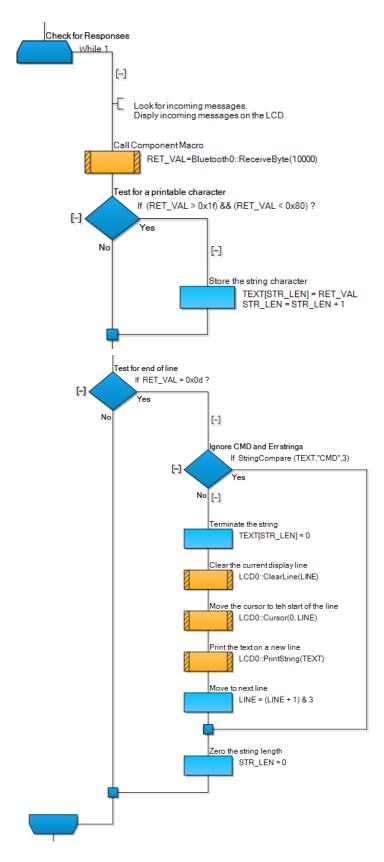
Once the inquiry has been sent the next step is to listen for responses. There can be a number of responses, so a loop structure is needed to go through them all, which is done by entering a continuous "while 1" loop.
