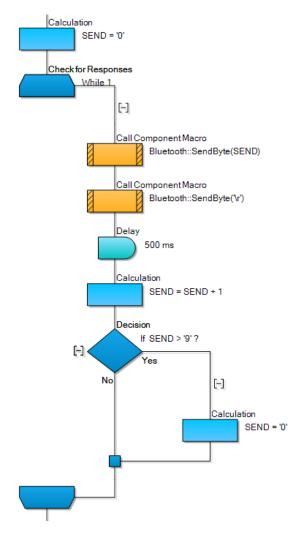
To demonstrate the connection is working a simple 0-9 repeating signal can be sent to be displayed on the receiving device.
