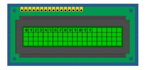
What we need to do is clear the LCD screen each time we write a new value. Luckily for us executing a clear screen routine also moves the cursor position back to (0,0). Add another component macro above the PrintNumber macro, and configure it to 'Clear'. We have now finished our third and final example. You should first test your program is right by comparing it to the code listing below. Simulate, before downloading to hardware to
